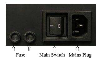
Fuse 2 Fuse holders for 5x20mm Fine Fuses 10A / delay type
