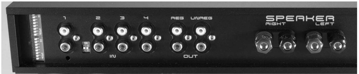
↑ Phono Adapter    ↑ Kanal 1 (Phono)    ↑ Kanal 2 (CD)    ↑ Kanal 3    ↑ Kanal 4    ↑ Regulatet Output    ↑ Unregulatet Output    ↑ Right    ↑ Left
